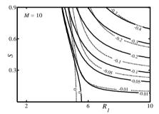
Figure 7. Variations of the modification friction factor normalized with the smooth annulus friction factor as a function of the cylinder curvature  $R_1$  and the groove amplitude *S* for M = 10 equal-depth trapezoidal grooves placed at the inner cylinder. Dashed lines are for the sinusoidal grooves with the same amplitude.
