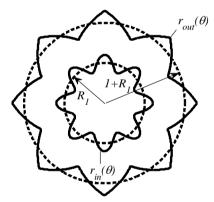
Figure 1. Sketch of the flow geometry - annulus with longitudinal grooves with an arbitrary geometry.
