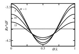
Figure 4. Distribution of the axial component of shear stress acting on the fluid at the outer cylinder. Other conditions as in Fig.3.
