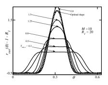
Figure 8. Evolution of the optimal shape of the unequal-depth grooves placed at the outer cylinder as a function of the depth of the groove  $S_{out,o}$ . The height of the groove is set at  $S_{out,i} = 0.5$ , M = 10 grooves are used
