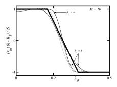
Figure 6. Evolution of the optimal shape of M = 10 equal-depth grooves placed at the inner cylinder as a function of the wall curvature  $R_I$ . Solid, dashed and dotted lines correspond to the depth of the grooves  $S_{in,i} = S_{in,o} = S = 0.2, 0.5, 0.8$ , respectively. Thick lines describe the universal shape, i.e. trapezoid with  $a = b = \lambda/6$  and  $c = d = \lambda/3$ .
