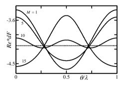
Figure 3. Distribution of the axial component of shear stress acting on the fluid at the inner cylinder for the same geometry as in Fig.2 but with the inner cylinder fitted with M = 1, 5, 10, 15 grooves. Dashed line provides reference value for the smooth cylinders.
