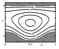
Figure 2. Distribution of the axial velocity component in an annulus with the inner cylinder with the average radius  $R_1=5$  fitted with five sinusoidal grooves with the amplitude  $S_{in}=0.3$  and a smooth outer cylinder.
