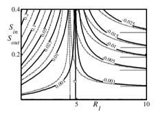
Figure 5. Variations of the modification friction factor normalized with the friction factor for the smooth annulus as a function of the groove amplitudes  $S_{in}$  (inner cylinder) and  $S_{out}$  (outer cylinder) and the radius of the inner cylinder  $R_1$  for the groove geometry described by one Fourier mode for M = 15 grooves. Solid (dash) lines correspond to grooves placed only at the inner (outer) cylinder.
